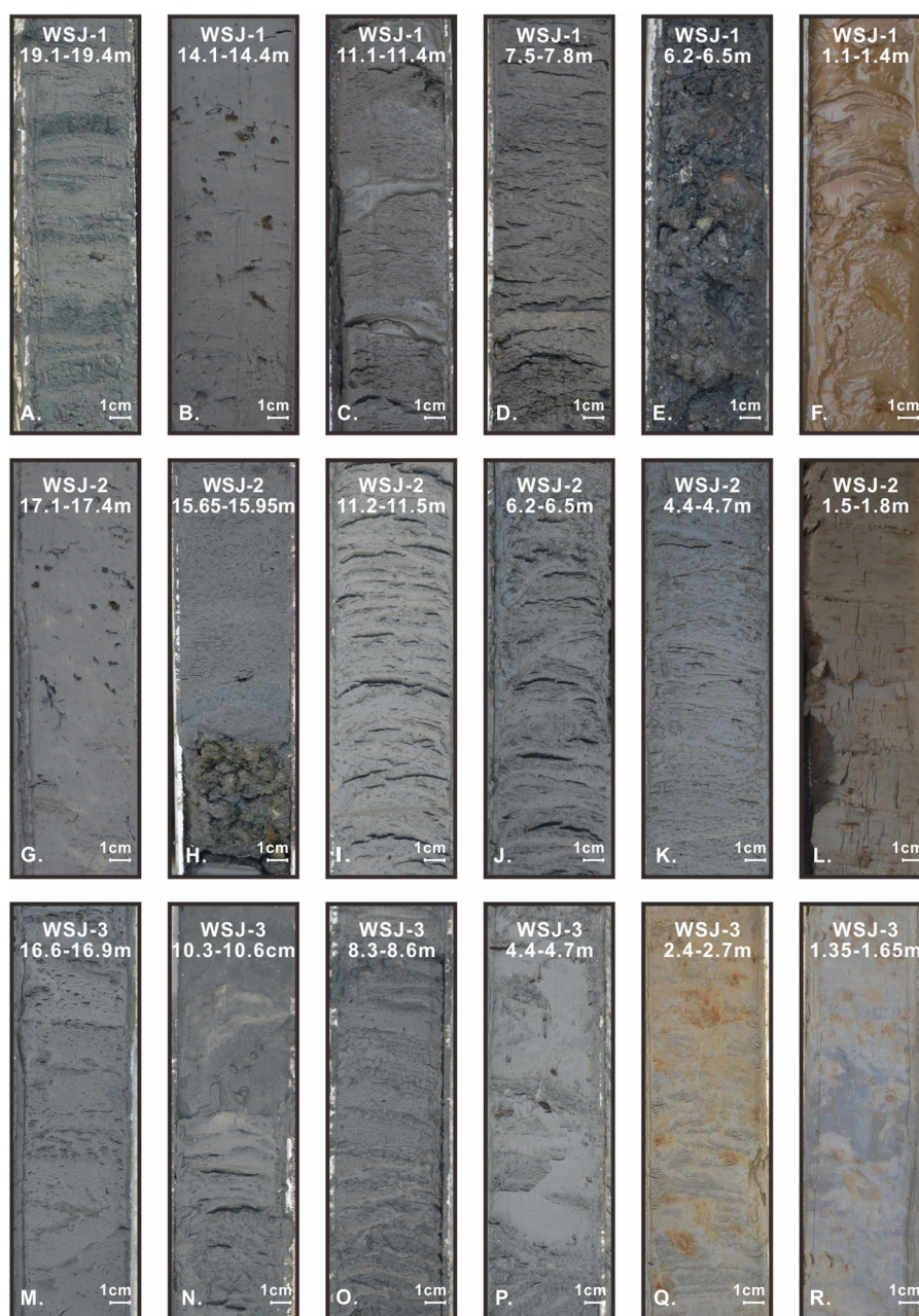
FIGURE 2 Photographs of typical lithological elements in cores WSJ-1 (A–F), WSJ-2 (G–L), and WSJ-3 (M–R). Note the various types of sand-mud couplets in each core.
