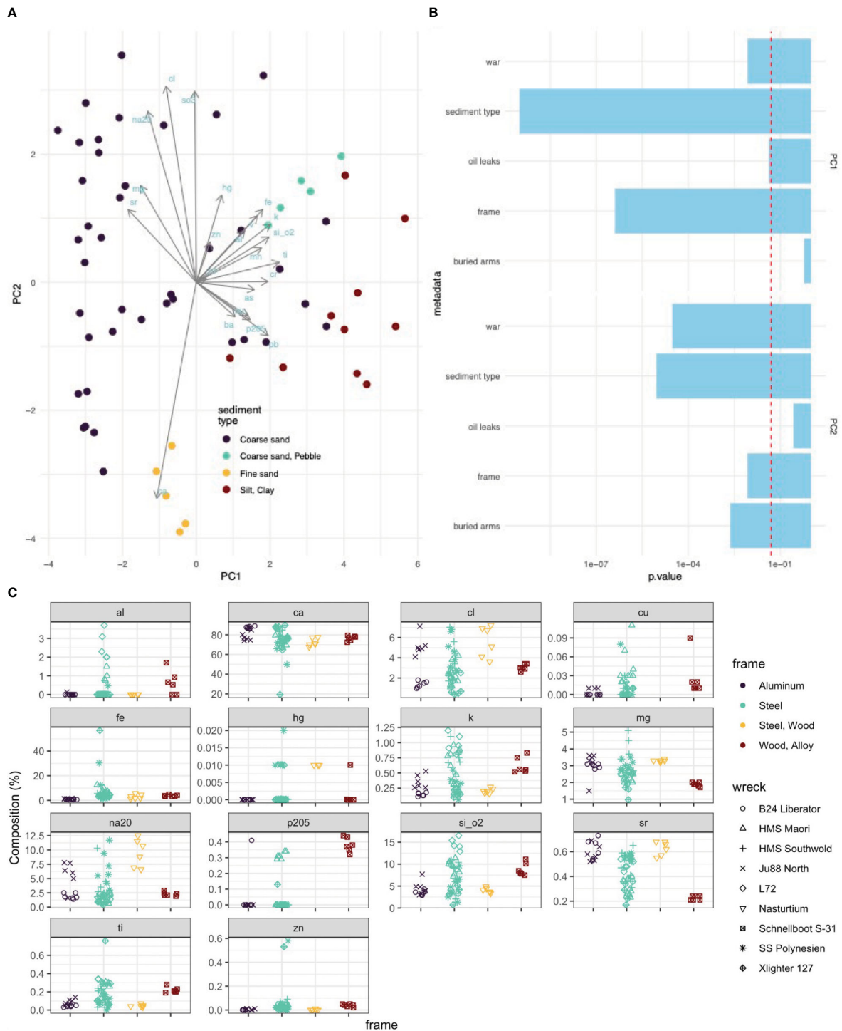
FIGURE 5 Chemical composition of the samples. (A) PCA (B) ANOVA of the categorical variables versus the two primary principle components. (C) Chemical composition data from XRF analysis of key elements associated with wreck material.
