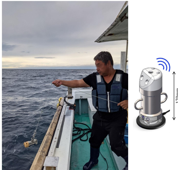
FIGURE 1 One fisherman just dropped S-CTD from his fishing vessel into seawater. The Bluetooth technology allows automatic transmission of measurement data to his Android device as soon as it returns above the sea surface.
