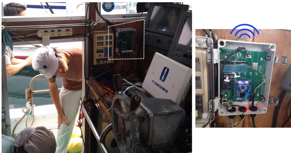
FIGURE 2 NMEA data logger (Yoron Denshi, Inc.) installed to a fishing vessel. This box records NMEA-0183 sentence including ADCP data from vessel electronic equipment(s) via wired serial connection. The data are then transferred wirelessly to an Android phone/tablet.
