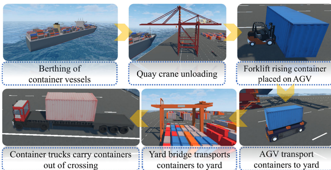
FIGURE 4 The process and the virtual model of hazardous cargo container imports in the port. Source: Models created with Unity, by the authors.
