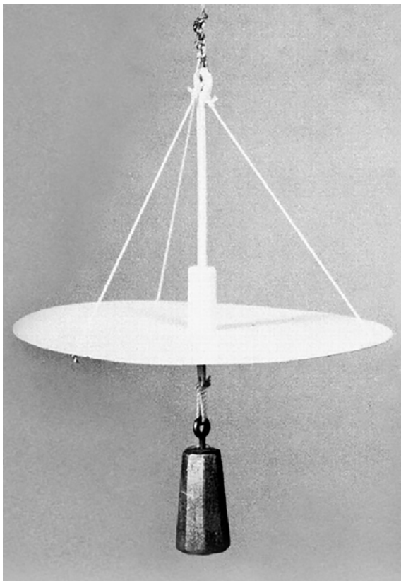
FIGURE 1 Illustrated example of a historical white-painted Secchi disk ( \varnothing = 45 cm) used on board the steamer “Pola” during the Luksch’s survey already around 1890 in the Red Sea and Mediterranean Sea (derived from Wernand, 2010).
