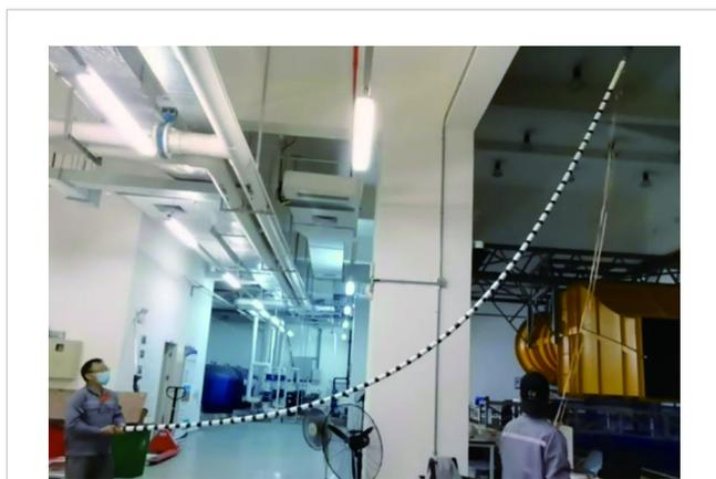
FIGURE 4 Hoisting of the riser model.
