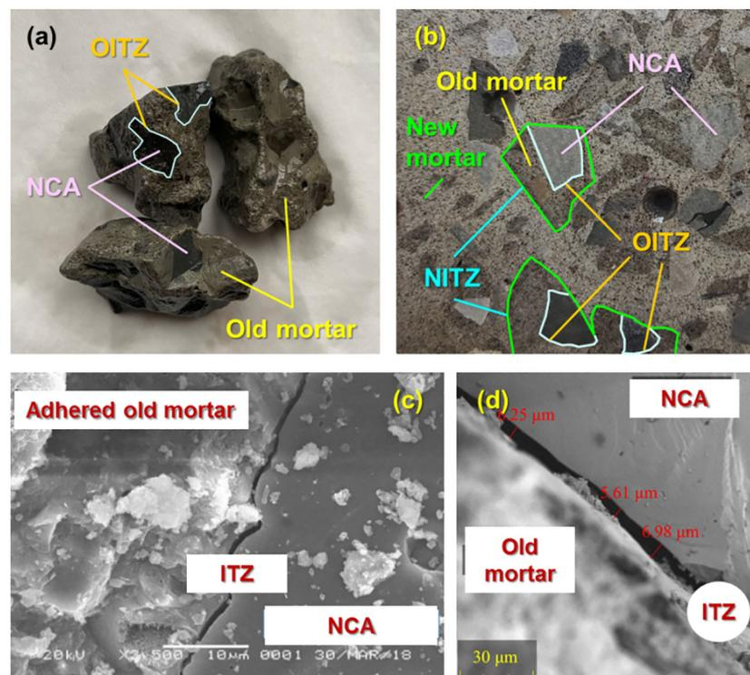
FIGURE 1 Mesoscopic structure of the (A) RA, (B) RAC, and (C) microstructure of the ITZ (Liang et al., 2019) and (D) microstructure of the ITZ (Li et al., 2020).
