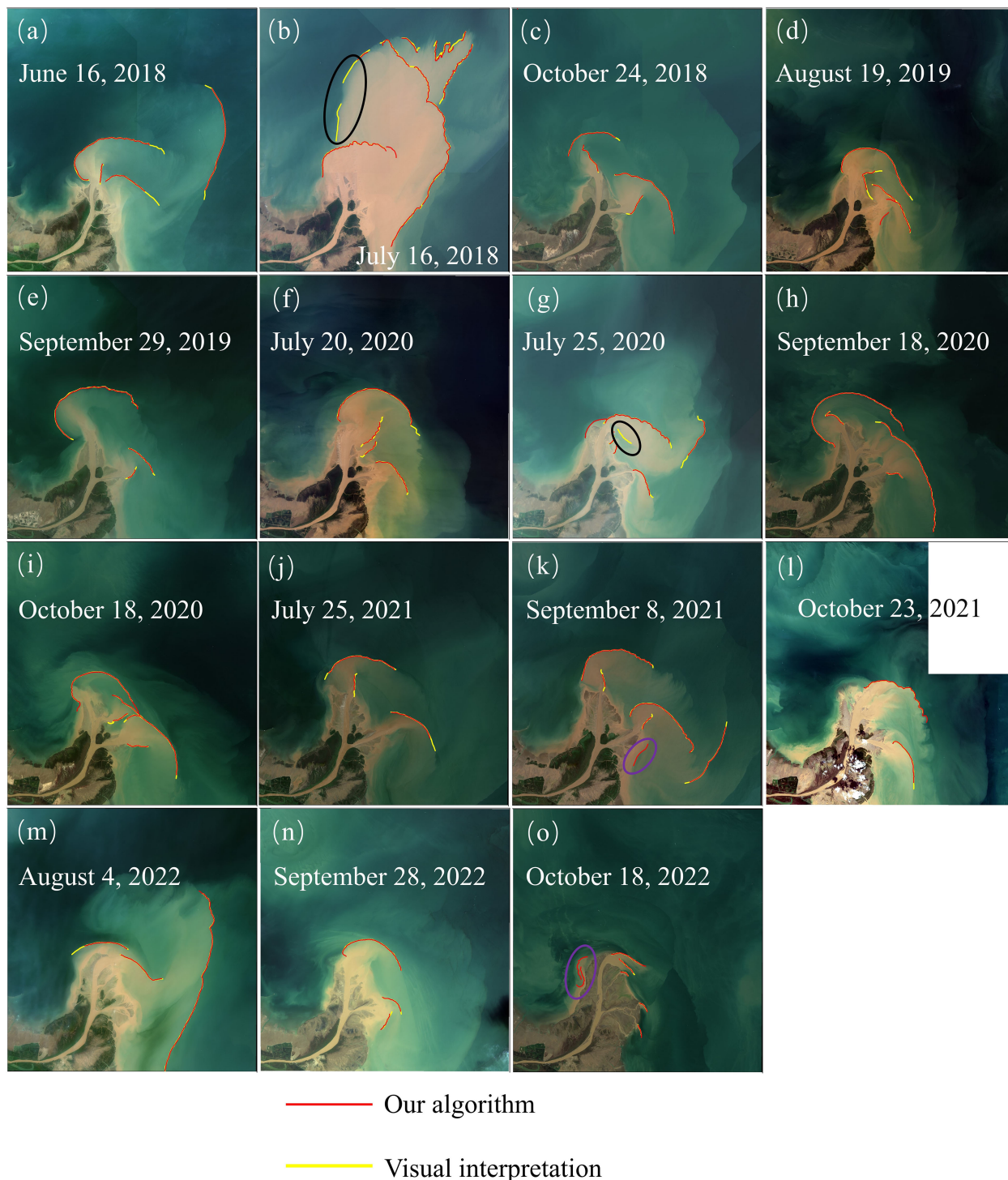
FIGURE 4 Presentation of YBDL distributions in the 15 randomly selected satellite images. The red lines were YBDL extracted by our algorithm and the yellow lines were YBDL outlined by manual visual interpretation. Those circled in black indicate missing YBDLs and those circled in purple indicate redundant YBDLs.
