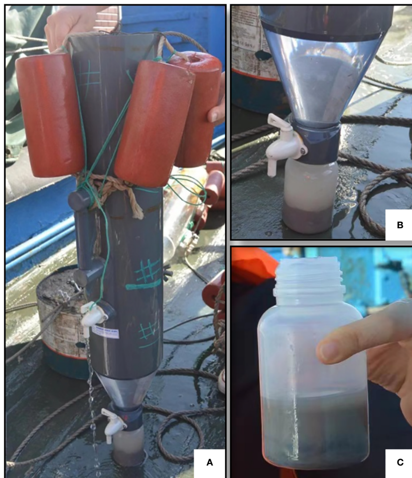
FIGURE 2 Photographs of sediment trap after retrieval. (A): supernatant water was released through the faucet; (B): collecting bottle; (C): trapped particles.
