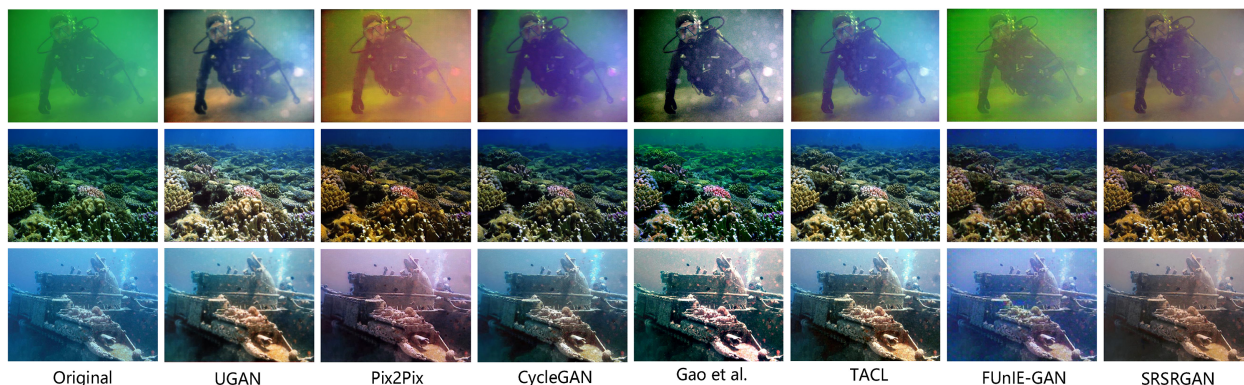
FIGURE 7 Qualitative comparison between SRSRGAN and the SOTA restoration/enhancement methods. From left to right are the original underwater images, the results of UGAN (Fabbri et al., 2018), Pix2Pix (Isola et al., 2017), CycleGAN (Zhu et al., 2017), Gao et al. (2019)'s method, TACL (Liu et al., 2022), FUnIE-GAN (Islam et al., 2020c), and SRSRGAN. Our sample image is sourced from the public dataset UIEBD (Li et al., 2020).
