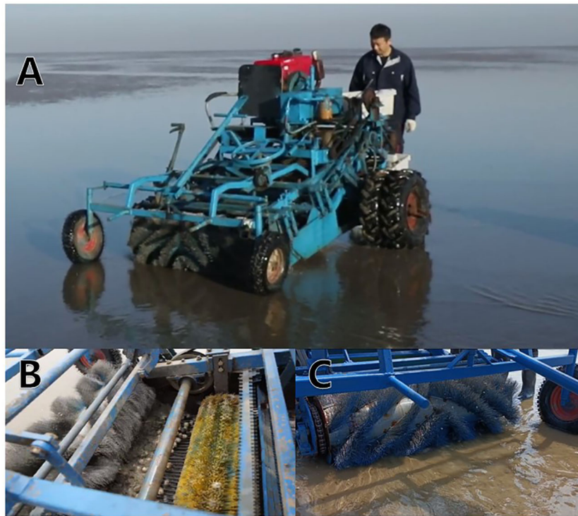
FIGURE 10 Shellfish vibration harvesting test: (A) The equipment harvesting operation, (B) The shellfish vibrating screening, (C) First-stage brush sediments cutting operation.
