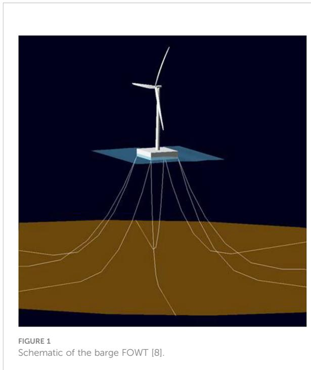
simplified dynamic model with limited DOFs is generalized for application in the design of TMD for FOWTs. Therefore, in this study, a simplified dynamic model of a barge FOWT with an MTMD was established to optimize the MTMD.
