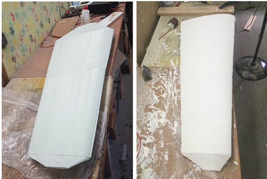
FIGURE 7 Foam wing glued together after manufacturing the single parts. In the right picture the application of the filler coat is depicted.
