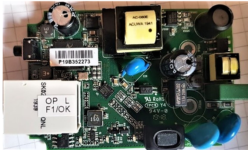
FIGURE 13 Front side of the power line adapter which was adapted and implicated into the system.
