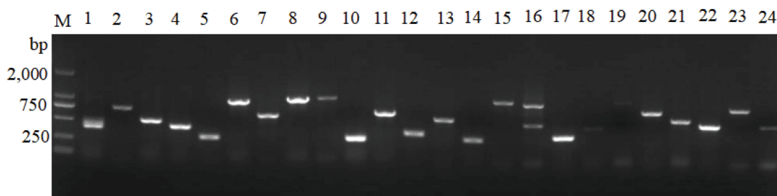
FIGURE 9 | Identification of the integrity of the recombinant sequence of the cDNA library. M: DL 2000 Marker. 1–24: PCR verification of positive colonies. Positive colonies were selected to evaluate recombination efficiency by PCR amplification with primers T7 and 3'AD.
