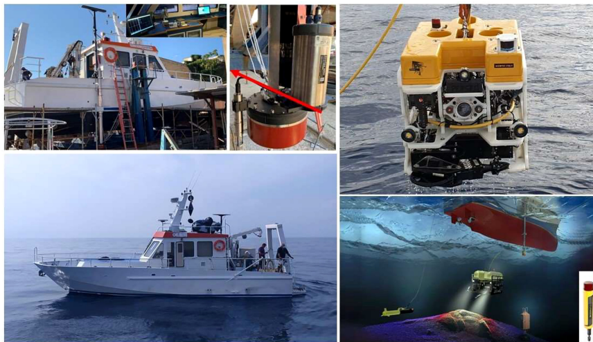
FIGURE 11 | M/V Lighea equipped with Kongsberg EM 2040 Compact Multibeam Echosounder Systems (MBES). ROV Perseo equipped with Kongsberg PAP 200 series USBL systems.
