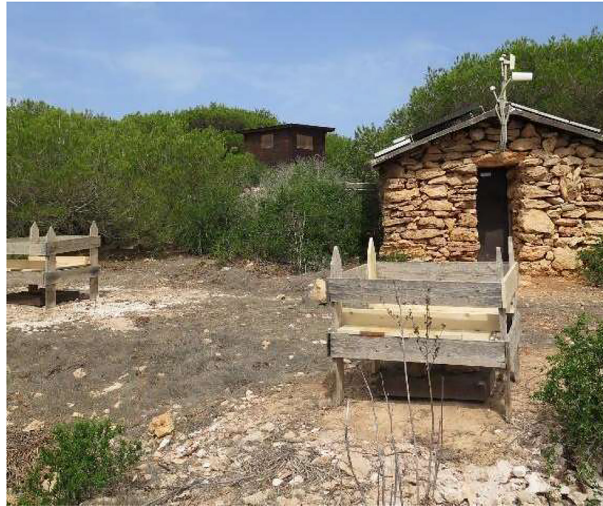
FIGURE 10 | Lampedusa Island Geophysical Observatory. The stone hut, due to its non-magnetic properties, is dedicated to absolute magnetic measurements, while the two fences protect the buried geophysical sensors.
