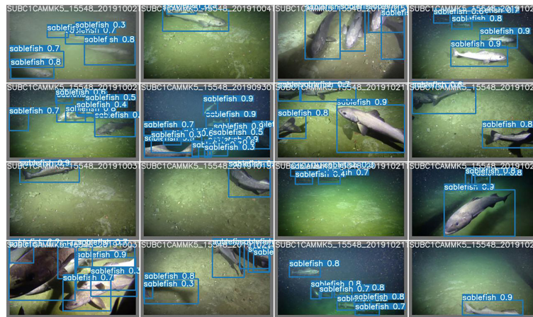
FIGURE 4 Examples of sablefish detection and classification at Barkley Axis (NE Pacific), showing multiple pan positions (camera moving laterally) and multiple tilt positions (camera moving vertically). The algorithm had to work under multiple illumination and seafloor configurations.
