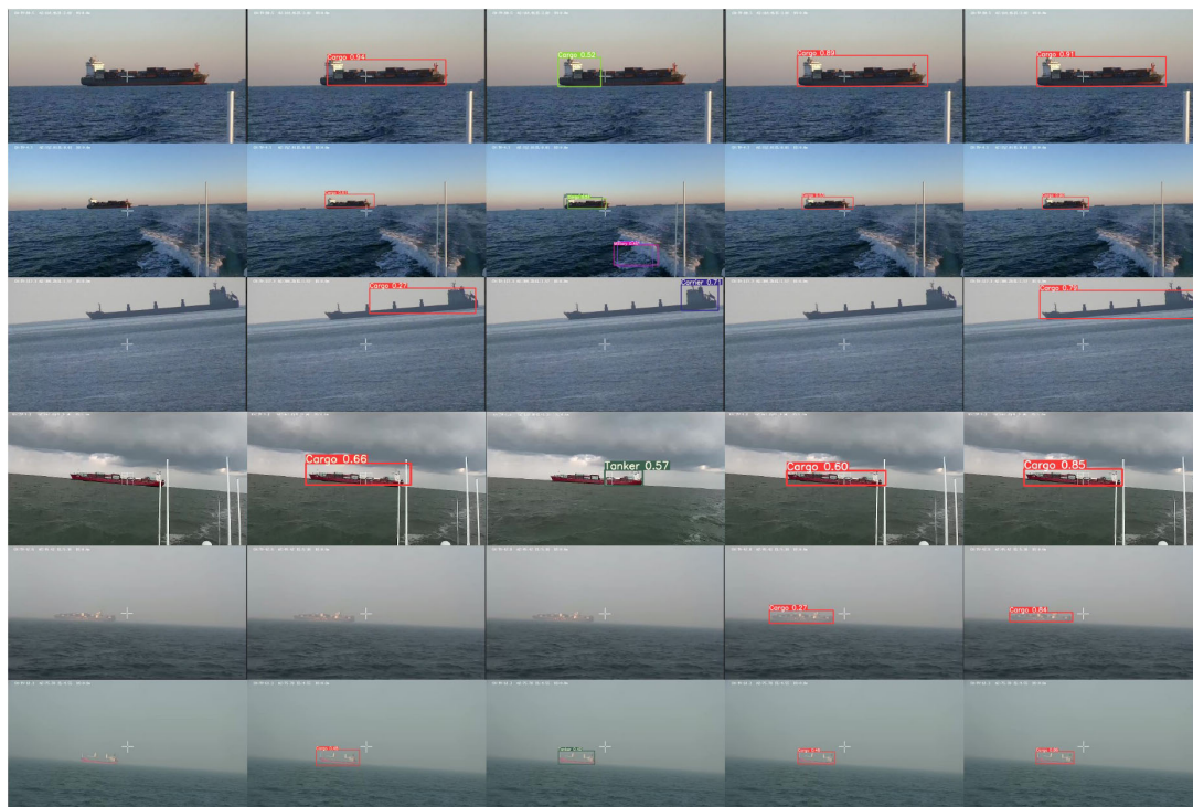
FIGURE 10 Detection results of different object detection algorithms in various environments collected by “JiuHang750” USV.
