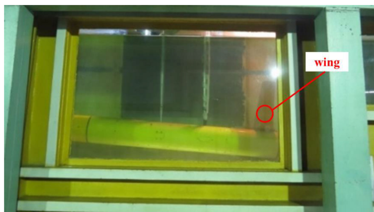
FIGURE 17 Equipment and glider in circulating flume test.
