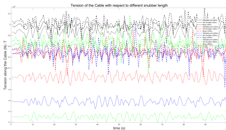
FIGURE 12 Dynamic tension for various components for different lengths of snubber for a Nilspin cable with the snubber up.
