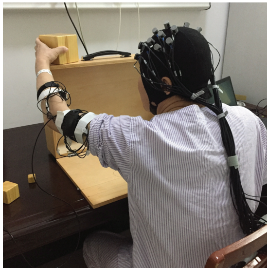
FIGURE 2 The illustration of fNIRS data acquisition.
