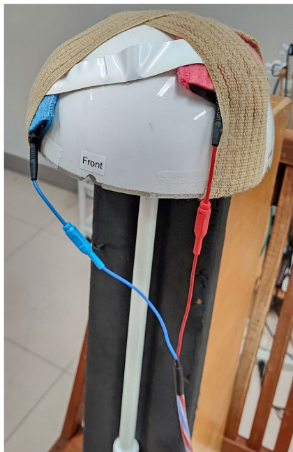
FIGURE 1 Setup of the phantom-tDCS experiments. Electrodes for transcranial direct current stimulation (tDCS) were fixed over the MEG phantom with rubber bands: the red electrode is anodal; the blue electrode is cathodal. The white band between the electrodes is a gel electrode providing a path for the electric current.
