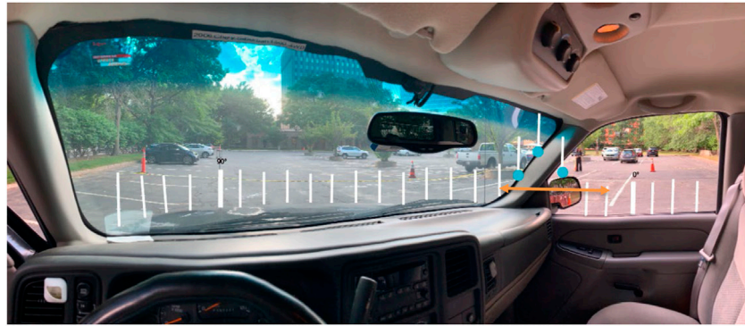
FIGURE 4 The non-visible points around the A-pillar in the forward seating position.
