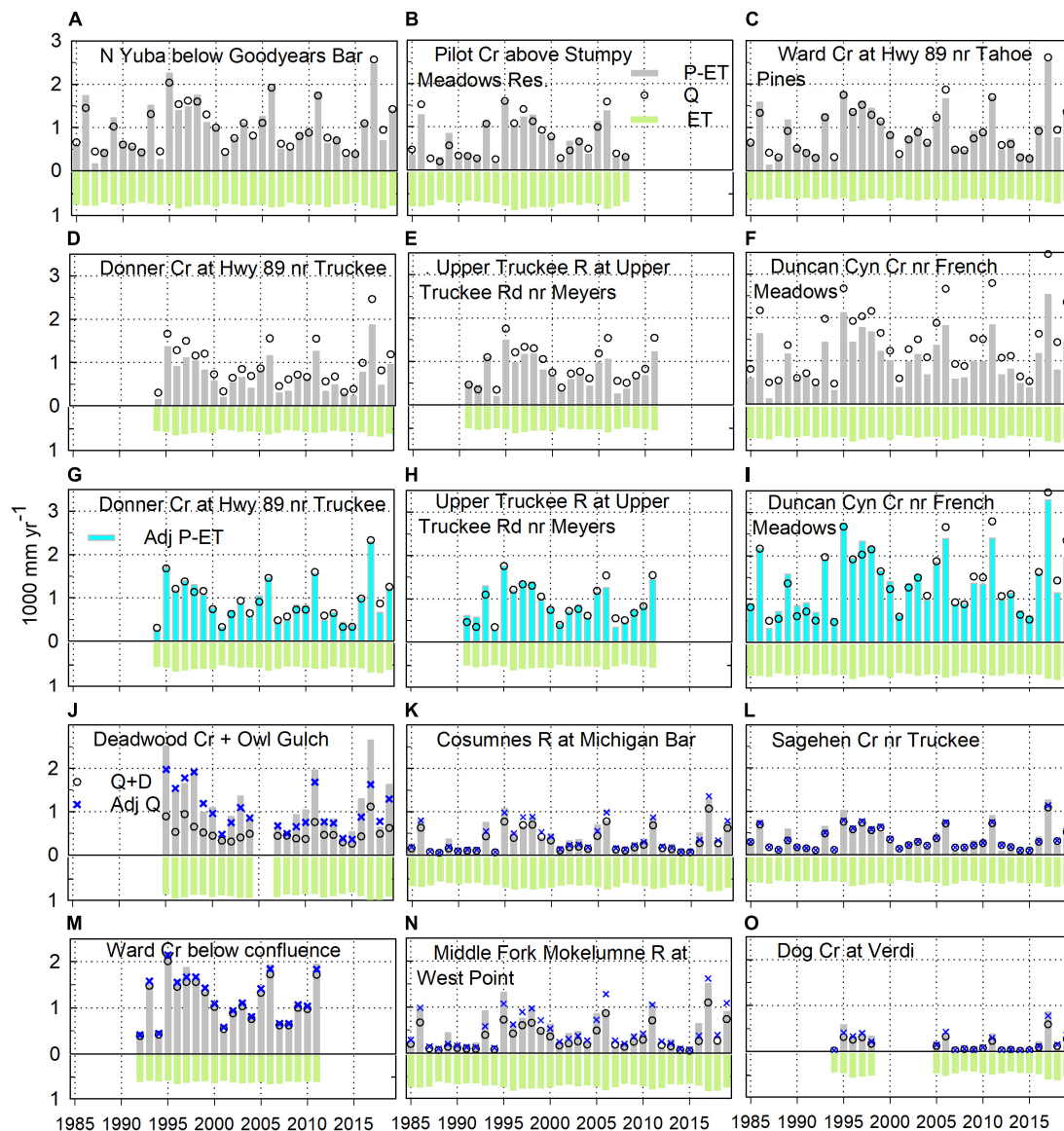
FIGURE 4 Water-balance time series for watersheds shown in Figure 3 (A–F) and Figure 5 (G–O). Note figure legends in (B,G,J).
