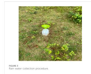
ensuring stability. Funnels were used to direct the water flow into the kegs. The kegs were monitored by the on-site field assistant to prevent the kegs from being displaced by the wind and to ensure adequate rain collection into the kegs while raining. The kegs were covered immediately after the rainwater collection and removed from their respective places.
