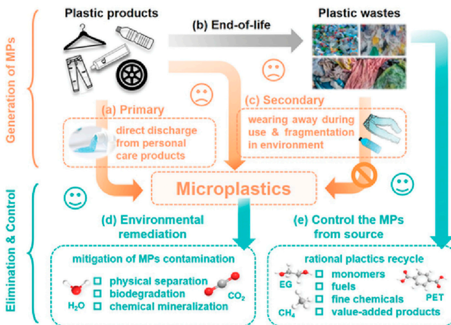
FIGURE 4 Microplastics production way, explain the process and management (Chen et al., 2022b).
