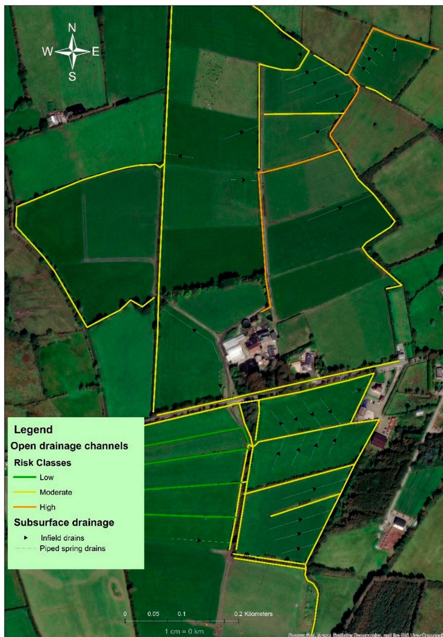
FIGURE 1 A map of a heavy textured grassland dairy farm (Farm #1 from Table 2) showing the risk classes of the open drainage channel network.
