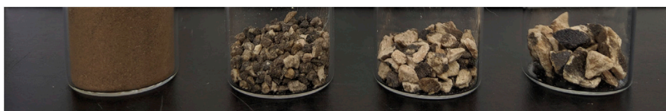
FIGURE 1 Image of Composition B particle sizes <2 mm (extra small), 2.00–2.83 mm (small), 2.83–4.75 mm (medium), 4.75–9.51 mm (large), from left to right.
