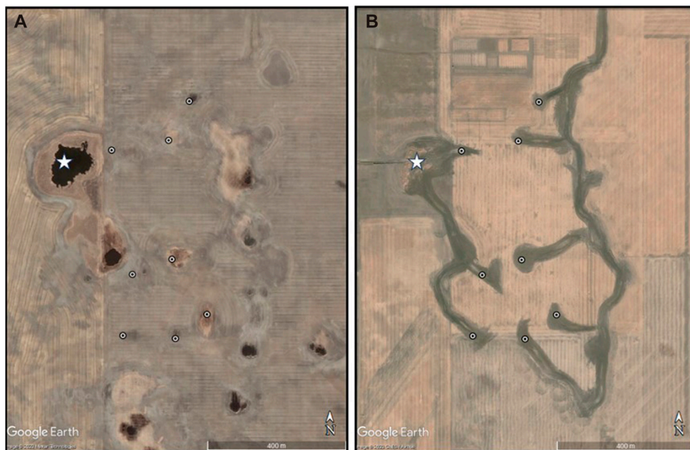
FIGURE 2 The wetland drainage complex at Discovery Farm in Langham, SK in (A) May 2014, and (B) October 2020. Wetland drainage ditches are observed in panel B as drainage was implemented in early October 2020. Drained wetlands are indicated by circles and the consolidation wetland is shown with a star. Imagery retrieved from Google Earth Pro, Google Earth Engine, Maxar Technologies, and CNES/Airbus.
