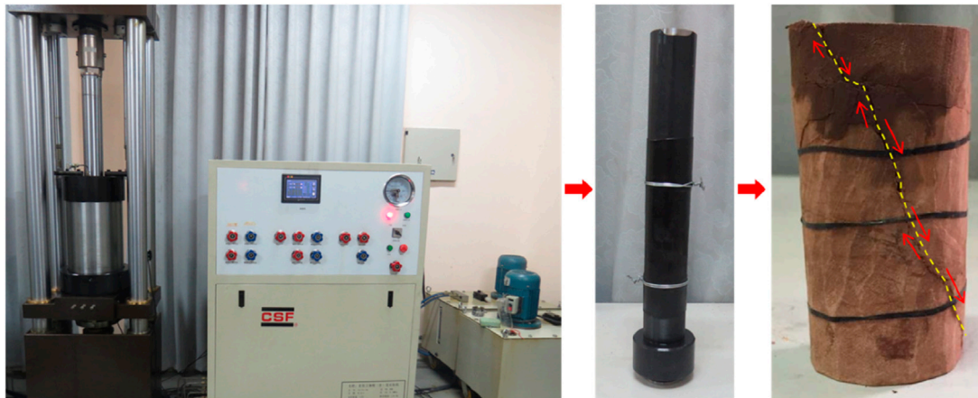
FIGURE 2 Experimental setup of the long-term creep test.
