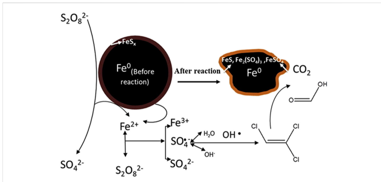
FIGURE 5 Possible degradation mechanism of TCE in S-ZVI/PS system. Adapted with permission from (Dong, et al., 2019a). Copyright 2019 Elsevier.
