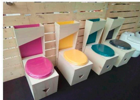
D Dry separation toilets used in the experiment.
