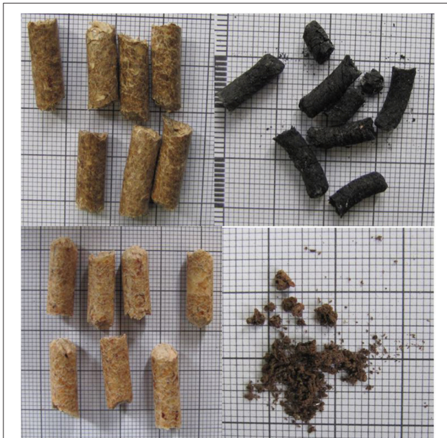
FIGURE 5 | Pellets before (left) and after (right) combustion at 900°C; t = 1,400 s; above: chaff pellets of fine fraction; below: pinewood pellets.
