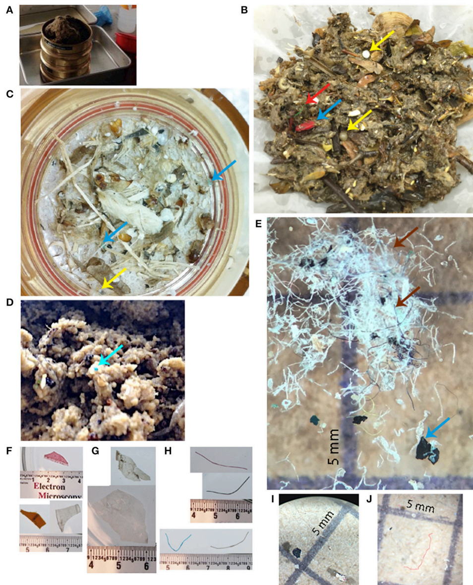
FIGURE 2 | Photographs of samples at various stages of processing, as well as examples of different shape classes. Arrows indicate plastic amidst co-sampled nonplastic organic matter; blue: fragment, dark red: line, yellow: nurdles, cyan: sphere/bead, brown: fiber. (A) Bulk sample directly upon retrieval from Manta on a stack of a series of sieves. This sample contained an abundance of algal biomass. (B) Bulk sample drying on a 53 \mu\text{m} mesh net. (C) Sample after enzymatic processing, which included an incubation in hydrogen peroxide that bleached much of the non-plastic organic matter. This bleaching aided in differentiating plastic (tended to retain color) from non-plastic (prone to bleaching) particles. (D) Examples of plastic of sphere class; zoomed in subset of sample in (B) . (E) Smallest size fraction (106–1,000 \mu\text{m} ) after WPO. Note colored plastic fibers (brown arrows) enmeshed in mass of natural fibers bleached white from hydrogen peroxide treatment. (F–H) Examples of plastic of fragment, film and line shape classes, respectively; ruler markings are in cm units. (J,I) Examples of plastic of paint chip and fiber shape classes, respectively; grid squares are in 5 mm units.
