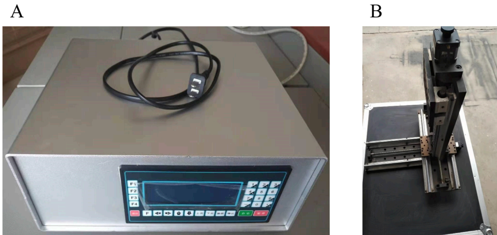
FIGURE 3 Probe control system: (A) 3D coordinate frame and (B) coordinate frame controller.
