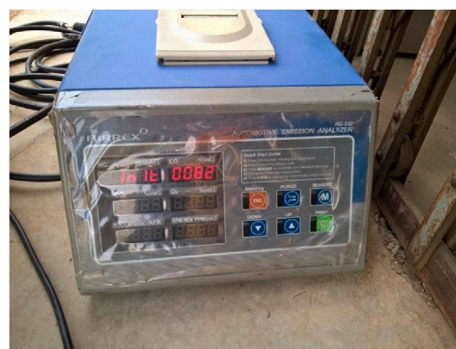
FIGURE 3 AIRREX HG-540 gas analyzer used to measure gas emissions.
