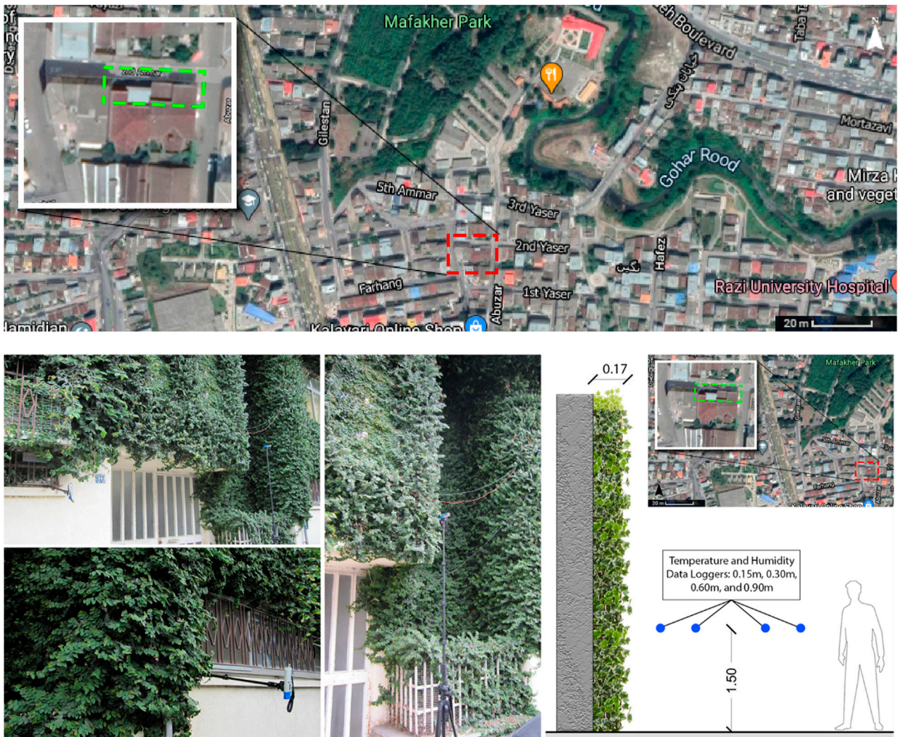
FIGURE 6 Layout of the study area and positions of data loggers for measuring ambient air temperature.
