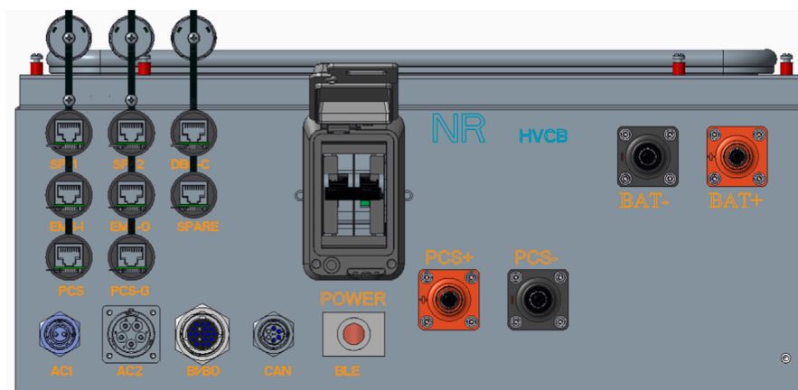
FIGURE 1 Schematic diagram of high-voltage box connection.
