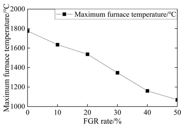
**FIGURE 9** The relationship between FGR rate and maximum combustion temperature.
