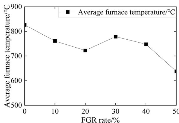
**FIGURE 10** The relationship between FGR rate and average combustion temperature.
