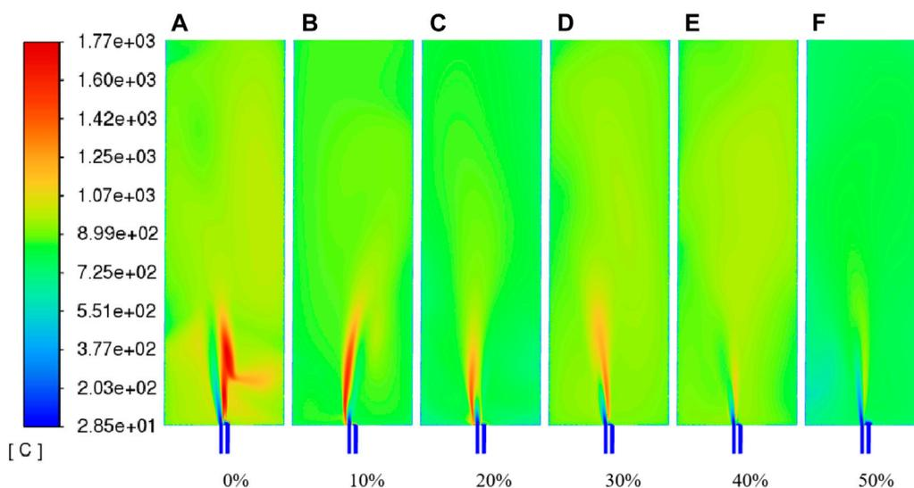
**FIGURE 8** Temperature field cloud images at different FGR rates: (A) 0% flue gas volume; (B) 10% flue gas volume; (C) 20% flue gas volume; (D) 30% flue gas volume; (E) 40% flue gas volume; (F) 50% flue gas volume.
