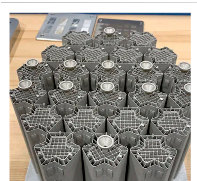
FIGURE 7 A fuel element featuring double-walled cladding and cooling channels that incorporate helical guides designed to enhance surface area. Credit: R. Dehoff, ORNL (DANIEL, 2020).
