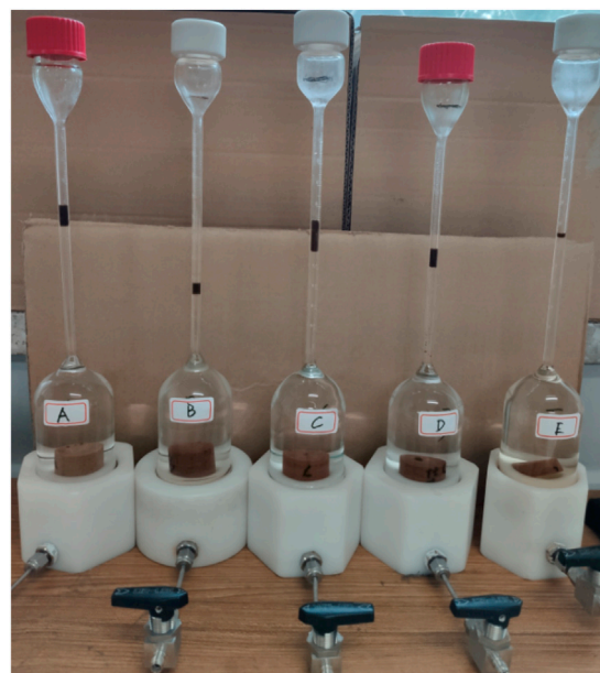
FIGURE 3 Amott spontaneous imbibition bottle during the experiment.
