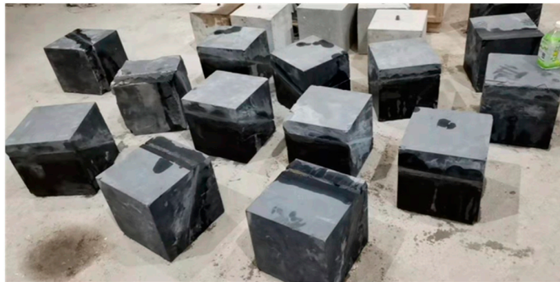
FIGURE 3 Production of shale rock samples containing filled faults after molding.
