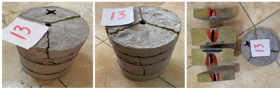
FIGURE 13 Fracture propagation diagram of No.13 shale rock sample.
