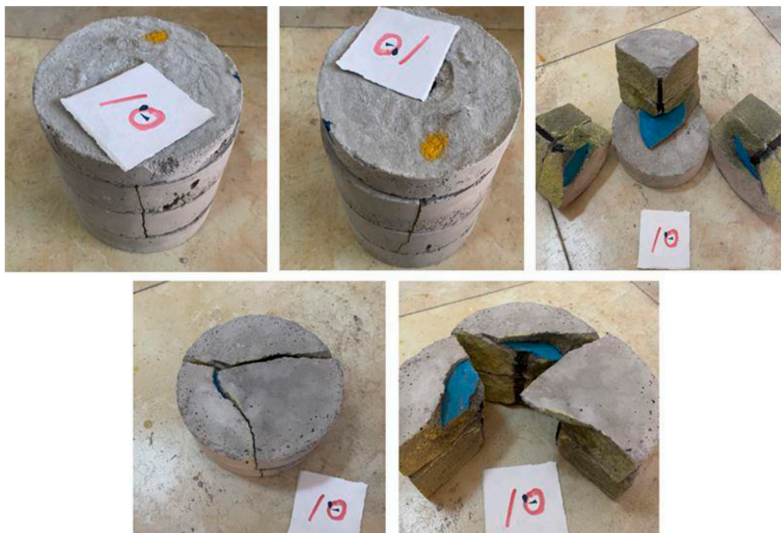
FIGURE 10 Fracture propagation diagram of No.10 shale rock sample.
