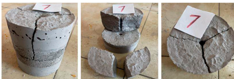
FIGURE 7 Fracture propagation diagram of No.7 shale rock sample.
