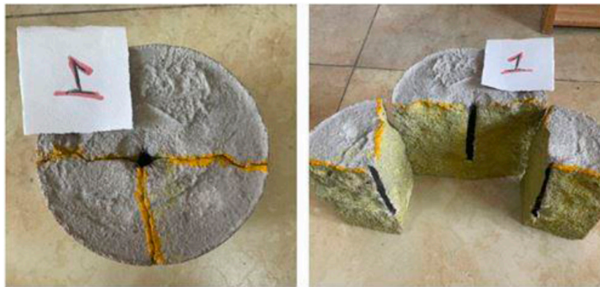
FIGURE 3 Fracture propagation diagram of No.1 shale rock sample.
