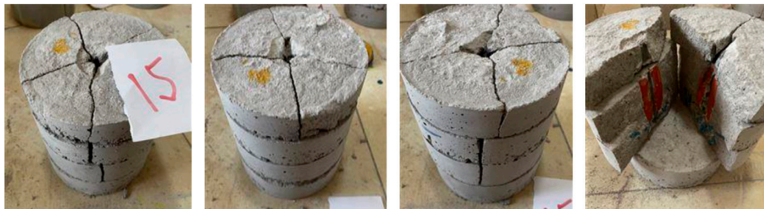
FIGURE 15 Fracture propagation diagram of No.15 shale rock sample.
