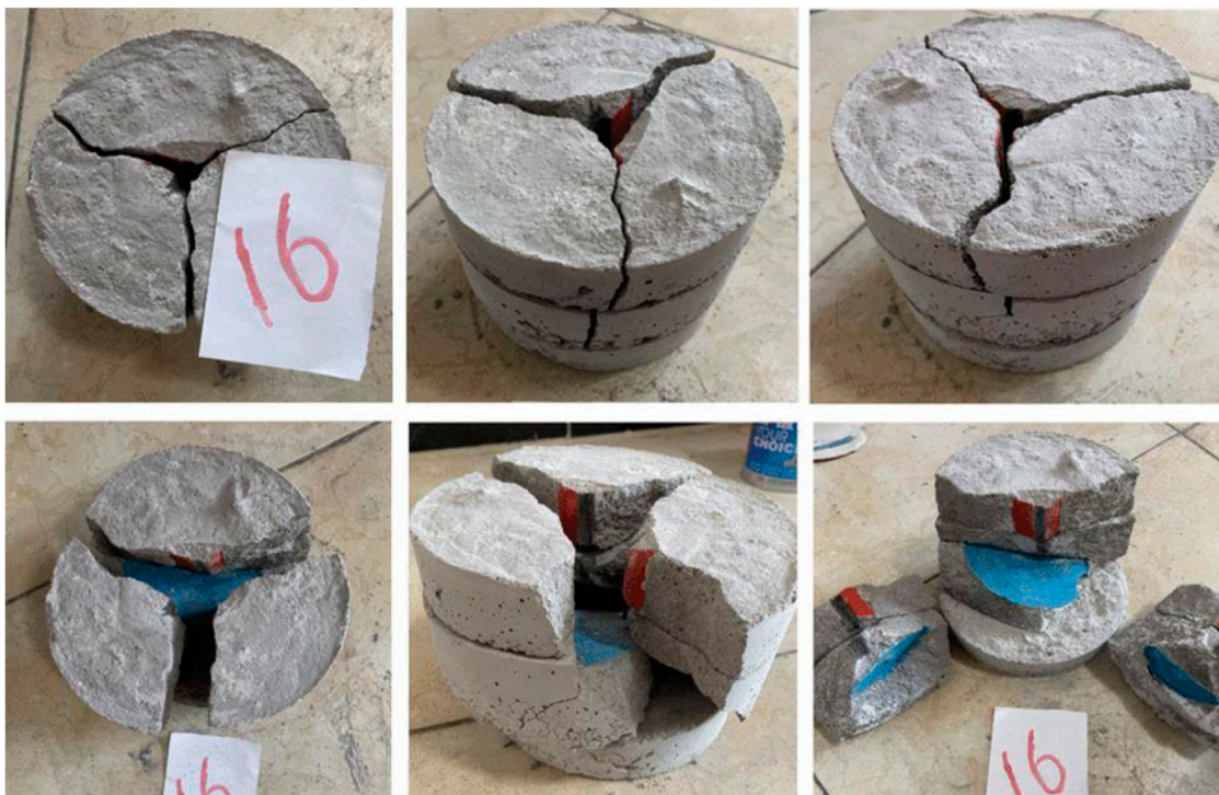
FIGURE 16 Fracture propagation diagram of No.16 shale rock sample.
