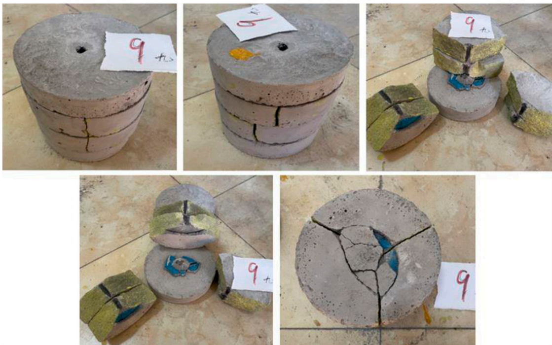
FIGURE 9 Fracture propagation diagram of No.9 shale rock sample.
