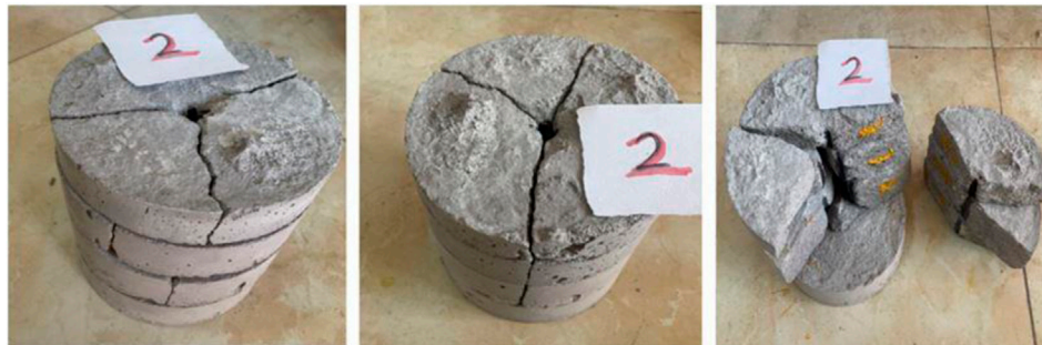
FIGURE 4 Fracture propagation diagram of No.2 shale rock sample.
