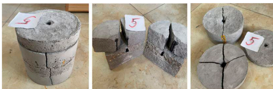
FIGURE 5 Fracture propagation diagram of No.5 shale rock sample.
