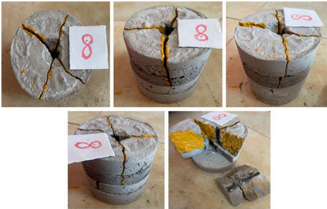
FIGURE 8 Fracture propagation diagram of No.8 shale rock sample.
