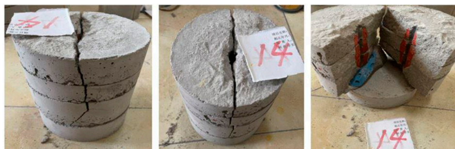
FIGURE 14 Fracture propagation diagram of No.14 shale rock sample.
