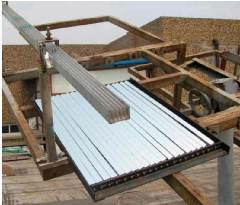
FIGURE 6 Picture of the linear Fresnel reflection solar concentrator photovoltaic experimental system.
