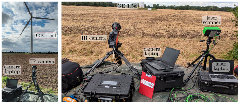
FIGURE 7 Measurement setup. Left: Positioning of the infrared camera downwind of the wind turbine in operation. Right: Measurement system consisting of an infrared camera (left, red) and a terrestrial laser scanner (right, green) plus a battery as mobile power supply as well as one measurement laptop for each device.
