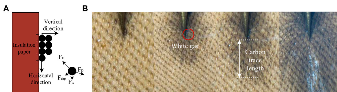
FIGURE 9 Carbon trace development process on cardboard surface in insulating oil containing carbon particles: (A) Schematic diagram and (B) Physical diagram.
