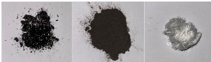
FIGURE 2 Experimental bio-ash and fiber materials (Left: carbon fiber; middle: bio-ash; right: alkali-free high-dispersion fiber).
