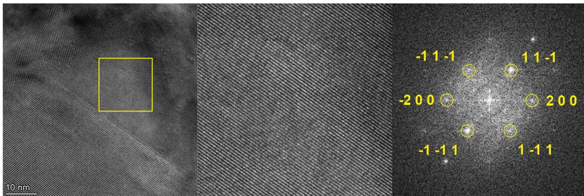
FIGURE 8 TEM bright field image of VN in high magnification, together with its FFT image showing a structure of VN (PDF#00-035-0768).
