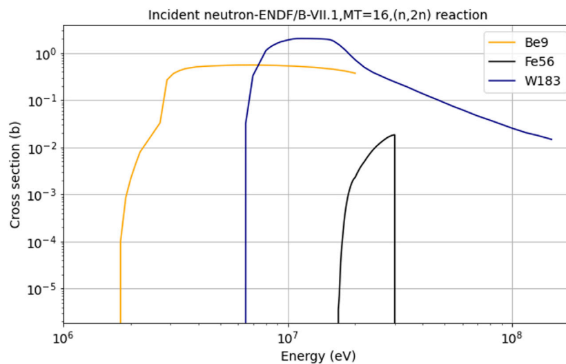
FIGURE 3 (n, 2n) reaction, MT = 16 cross-section distributions of 9 Be, 56 Fe, 183 W.
