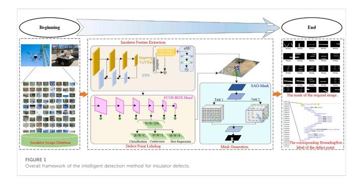
efficient extraction of target features. 2) The spatial attention-guided mask (SAG-mask) branch generates target masks. 3) Using fully convolutional one-stage (FCOS) to detect defect points of insulators. Finally, the end realizes the output of the insulator mask and the bounding box label of the defect point.
