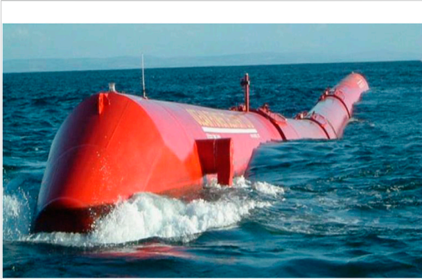
FIGURE 4 Pelamis wave energy conversion device (Yemm et al., 2012)
